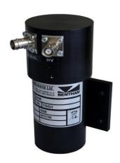
The DH\_30 photomultiplier is an economical solution for low light-level applications throughout the UV-vis. Housing a side-window multi-alkali (S20 photocathode) photomultiplier tube, a mu-metal shield and a PCB based dynode chain, reliable operation can be ensured. The 215 high voltage supply module maintains the photocathode at a negative high voltage.
